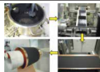
Figure 52 : Images of (a) 2.5 kg of slurry contains LTO, binder and carbon black and (b-d) coating, drying and roll of large scale synthesized LTO electrode fabricated by Li-ion pilot plant unit.
